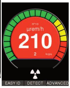
The Detect measuring mode is a tool to locate radiation sources by giving rapid visual and audio feedback to the changing dose rate of incoming radiation. After switching to Detect mode, the user can localize the radiation source by monitoring (in real-time) the auto-scaling chart with color enhanced areas representing the dose rate history of the last few seconds. When the source has been localized, the user may then initiate an "Easy ID" to quickly identify radiating nuclides.
