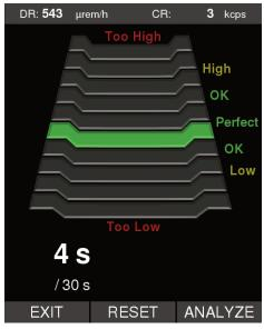
In Easy ID mode, the RADEAGLET-R acquires a spectrum. The screen at left is used to find an optimal position to ID the source. The user can preset duration if desired, then analyze and save the results. During the acquisition, an on-screen chart instructs the user to find the best distance between the instrument and the source in question. The nuclides identified will be displayed. The recorded spectrum and the analysis results are saved to an internal SD card in ANSI N42.42 format.
