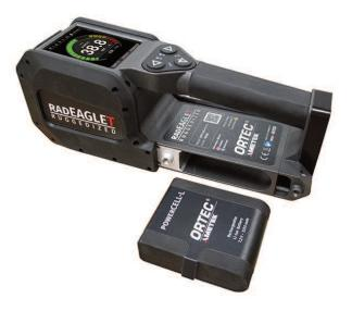
RADEAGLET-R has a small internal rechargeable battery which keeps the system running for a short period of time without any external power. This gives the user several minutes to change the battery pack without needing to switch the unit off and on.
